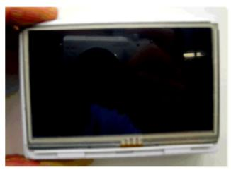
Connect communications cable to rear of screen, and clip screen into cover mounted in wall.
